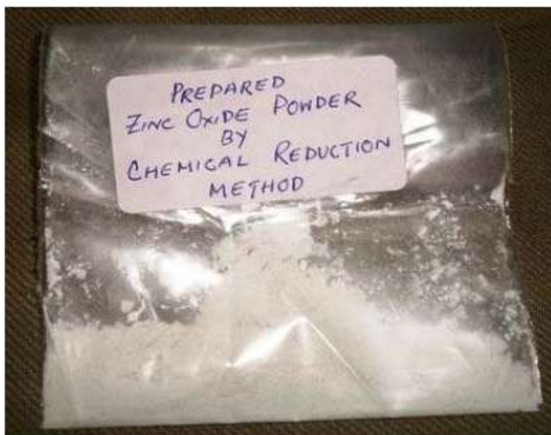
Figure 3. Synthesized ZnO powder by chemical reduction method
